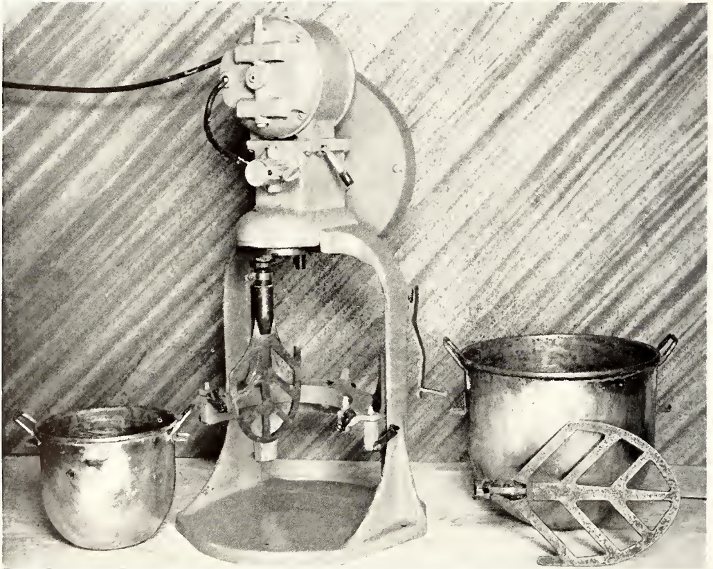
FIGURE 5-10—Three-speed, dough-type, electric mixer equipped with 3- and 8-quart bowls and two sizes of paddles for mixing glues.
